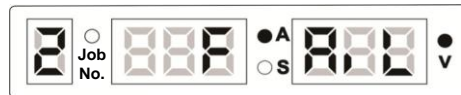
Figure 3-30 Message indicating that the confirm password is different from the new password
