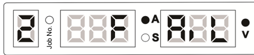
Figure 3-33 Message indicating that the confirm password is different from the new password
